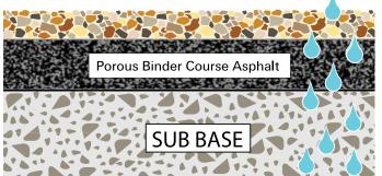
Top surface: **15 -18mm** thick 'bound' mixture of stones and resin
