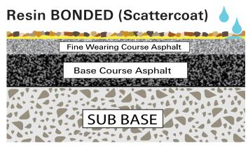
Top surface: **3mm** layer of single stones 'bonded' to resin
