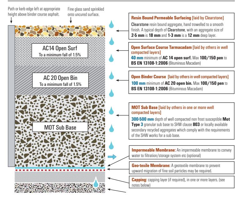
Please note: New asphalt and concrete surfaces need a minimum of <u>two weeks curing</u> time, before resin bound paving can be laid upon it.
