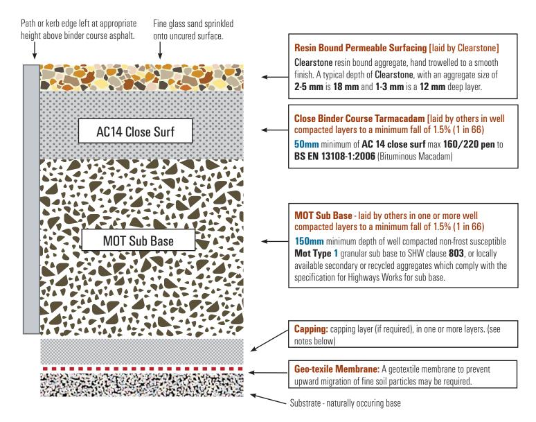
Please note: New asphalt and concrete surfaces need a minimum of <u>two weeks curing</u> time, before resin bound paving can be laid upon it.
