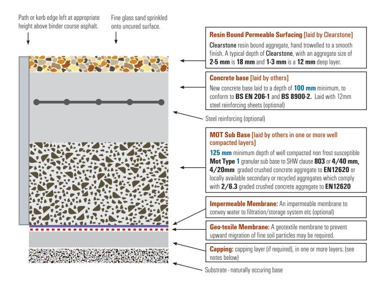
Please note: New asphalt and concrete surfaces need a minimum of two weeks curing time, before resin bound paving can be laid upon it.
